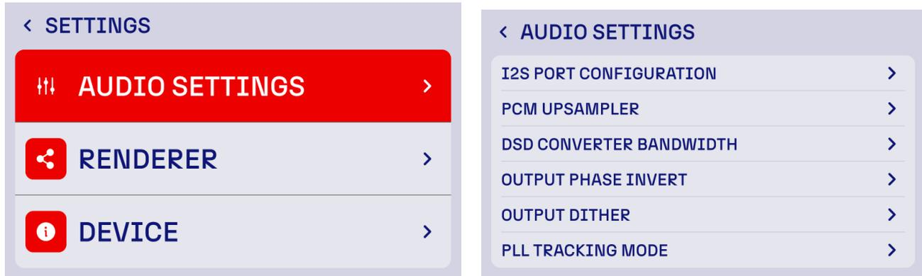
In the settings menu, the following options will be available, I2S port configuration, PCM Upsampler, DSD Converter Bandwidth, Output phase inverter, Output Dither and PLL Tracking Mode. Touch to access the desired settings submenus.
